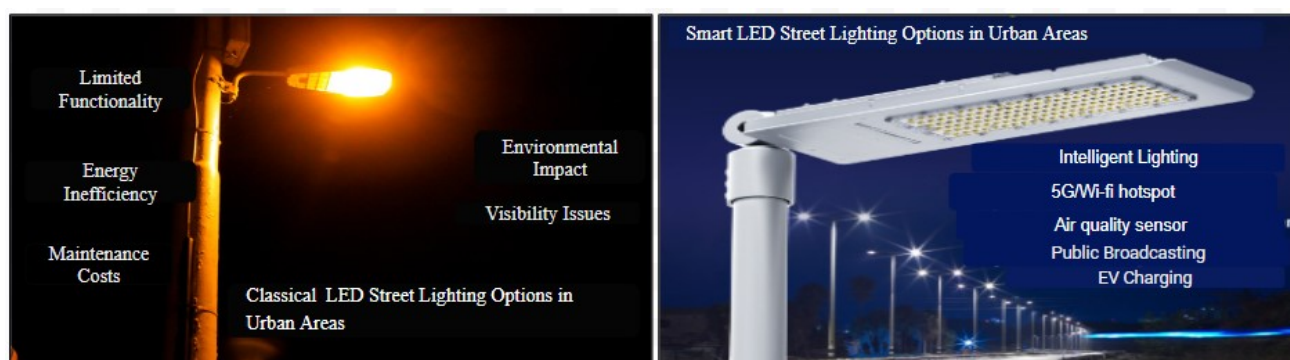
Fig. 1. Comparison between Classical and Smart LED Street Lighting in Urban Environments [9, 10]
